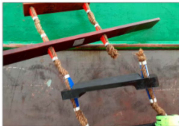
Figure 2: Example of a failed pilot ladder
