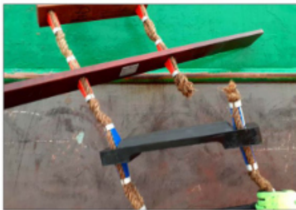
Figure 2: Example of a failed pilot ladder
