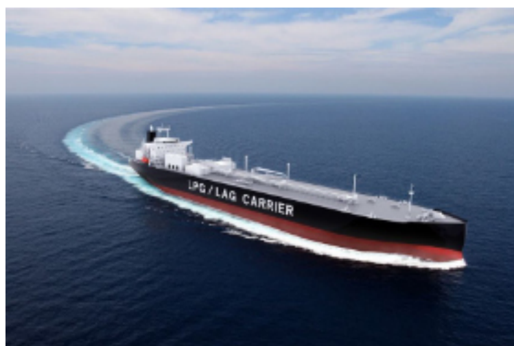
An ammonia-ready very large gas carrier (VLGC). (Illustration courtesy of Mitsubishi Shipbuilding Co Ltd. ©)
