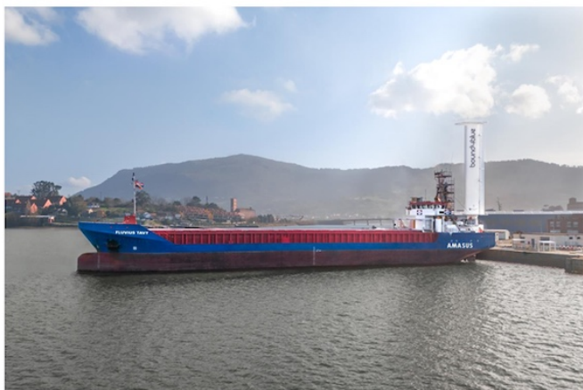
22-metre eSAIL® installed on Fluvius Tavy (Source: bound4blue)
