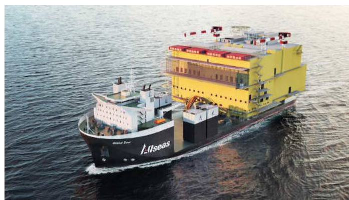
Semi-submersible heavy transport vessel Grand Tour. Image credit: Allseas ©.
